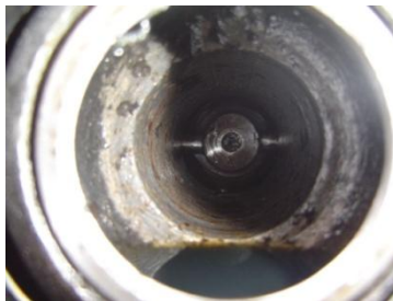
Figure 1 Crank Handle hole showing horizontal position of crankshaft pin at TDC.
